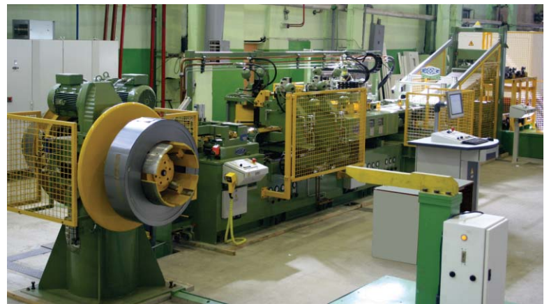
THE SLITTING AND CUT-TO LENGTH LINES FOR ELECTRICAL STEEL (GEORG COMPANY)
