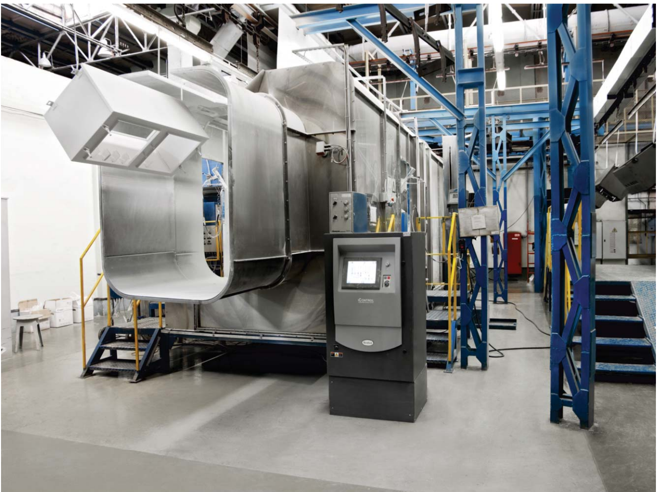
POWDER COATING LINE OF NORDSON (USA) AND ZYGIL COMPANY (POLAND)
