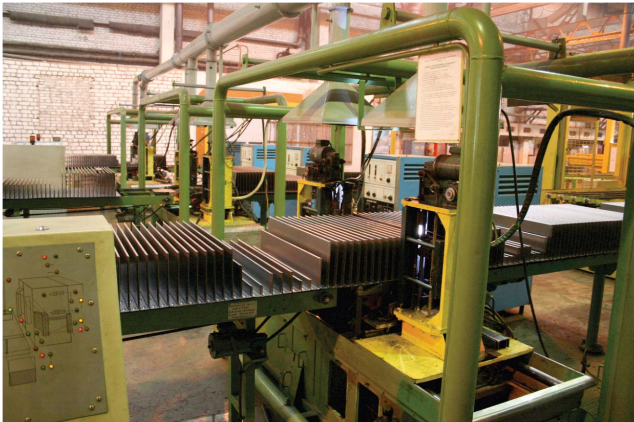
LINE FOR PLASMA WELDING OF CORRUGATED WALLS
